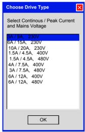
When you have selected the servo drive type, a default data set is loaded. This data can be modified and stored in an external file.
