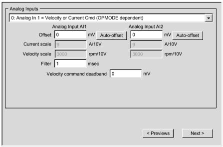
Cycle time of the Analog Input functions: 250 micro-seconds. Analog Input Al1 is read every 125 micro-seconds.
