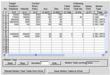
A Motion Task may be started by a Digital Input or a field bus order.
