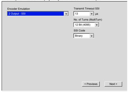
For information on wiring the Encoder Emulation Output on an X5 Connector, see the Lexium 15 LP Installation Manual.
