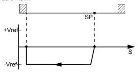
Homing to mechanical stop, **positive direction** of motion, positive rotation, without zero mark.
