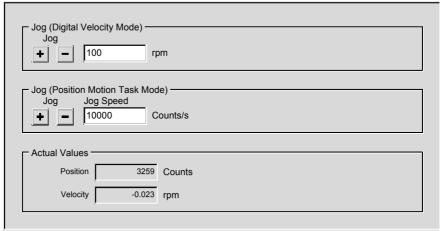
The drive moves with the preset speed when the + or – button is pressed. It stops when the button is released.
