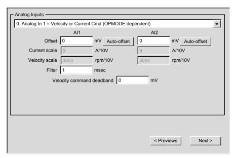
These functions are declined in fourteen variations, which are all described in detail in the Analog Inputs section (See *Overview of the Analog Inputs Screen, p. 148*). Click "Next" to move to the next screen in the Setup Wizard.
