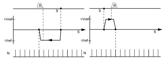
Homing with reference switch, negative direction of motion, positive rotation, with zero-mark.
