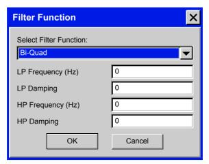
LP frequency field will fill in ARLPF (anti-resonance frequency) and HP frequency field will fill in ARHPF (resonance frequency).LP damping field will fill in ARLPD and HP damping field will fill in ARHPD. Setting all parameters to 0 disables the filter.
