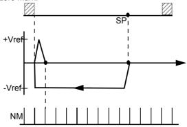
Homing to mechanical stop, **positive direction** of motion, positive rotation, with zero mark.
