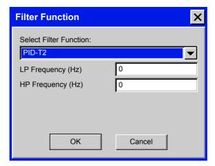
The LP frequency field will fill in ARLPF (anti-resonance frequency) and the HP frequency field will fill in ARHPF (resonance frequency).
