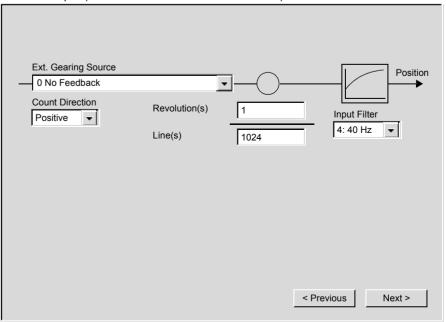
This screen is described in detail in the Electronic Gearing section (See *Overview of the "Electronic Gearing" screen, p. 136*). Click "Next" to move to the next screen in the Setup Wizard.
