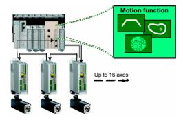
Multi-axes synchronised applications with Sercos Motion bus in TSX CSY 84/164/85 for Premium PLC:
