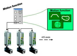
Multi-axes synchronised applications with CANsync Schneider standalone Motion Controller:
