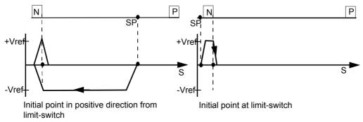
**Note:** Hardware limit-switches must be present and connected. The LI3 and LI4 digital input limit-switch functions 2, PSTOP and 3, NSTOP must be switched on.
