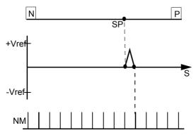
**Note:** behavior for successively repeated starts of Homing 5: the position controller can only hold the motor in the zero position by passing the zero mark by 1 count. On a repeated start of Homing 5, depending on the position (1 count in advance of or 1 count behind the zero-mark) and the count direction, the movement may be a full motor turn!
