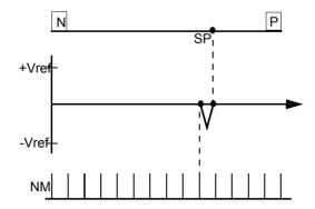
Homing with reference switch, **positive direction** of motion, positive rotation, with zero mark.
