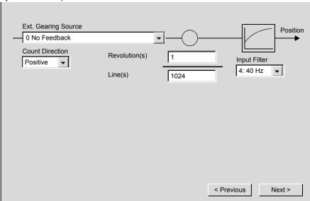
The servo amplifier receives a position setpoint from another instrument (master servo amplifier, stepper motor control, encoder or similar) and controls the position of the motor shaft in synchronism with this master (control) signal.
