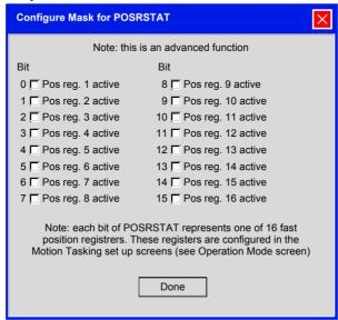
The bit mask is compared with the bit variable contents according to the selected logic (AND, OR,). The digital output is set if the result is a logical 1.
