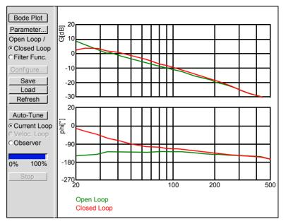
This screen displays the frequency response for speed control. The system is simulated using a sinusoid input variable. The output variable has identical frequency but different amplitude and is out of phase by several degrees.
