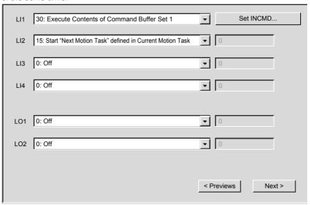
This screen is described in detail in the Digital I/O section (See *Digital I/O Overview*, p. 158). Click "Finish" to end the Gearing Application Setup Wizard.
