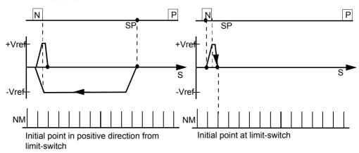
**Note:** hardware limit-switches must be present and connected. The digital inputs LI3 and LI4 limit-switch functions 2, PSTOP and 3, NSTOP must be switched on.
