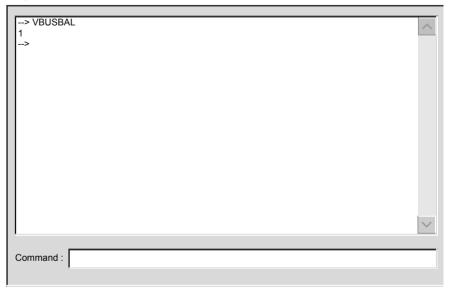
Communication with the servo amplifier is made through ASCII commands. You can obtain a complete list of the commands from our application department.
