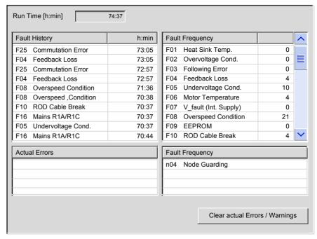
On the top left pane is the error history with the time (run time) when the error occured. On the top right pane information about the frequency of every error is listed. Below these frames, the actual errors and warnings are listed.
