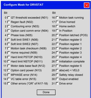
The bit mask is compared with the bit variable contents according to the selected logic (AND, OR, NAND, NOR). The digital output is set if the result is a logical 1.
