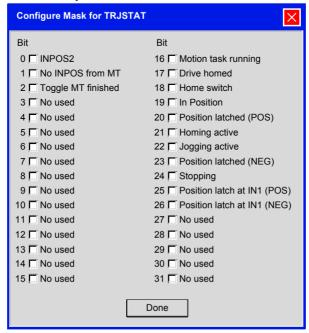
The status information 3...15 and 27...31 are primarily used for internal functions. Bits 0...2 and 16...26 can be used for external functions (control system).
