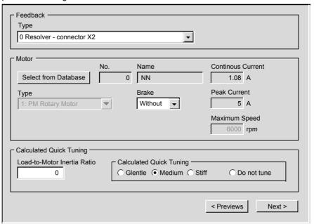
This screen is described in detail in the Motor/Feedback section (See *Overview of the "Motor/Feedback" screen, p. 92*). Click "Next" to move to the next screen in the Setup Wizard.
