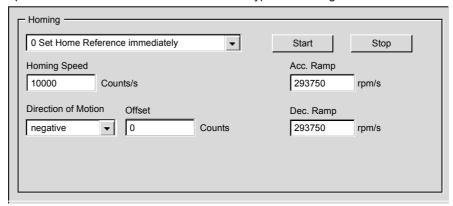
After homing, the drive reports "InPosition" and then enables the position controller in the servo amplifier.
