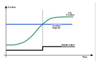
The position registers are configured using 3 control variables. The position signals are indicated through a status variable. All control/status variables can be considered as 32-bit variables, whereby the lower 16 bits (bits 0 ... 15) are used for the configuration of the position registers P1 ... P16.
