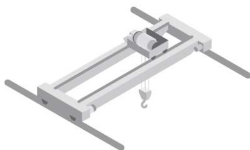
Machine with CANopen architecture: - Lifting motion: Altivar 71 - Translatory motion: Altivar 312 - Carriage motion: Altivar 312
